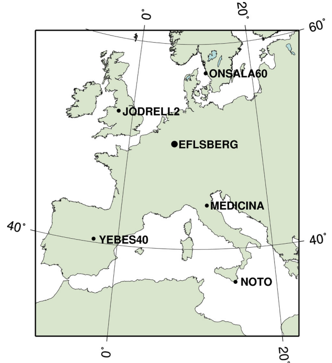
Figure 1. The EVN stations that participated in the EGaPS experiment. The longest meridional baselines NOTO/ONSALA60 is 2280-km long. The longest longitudinal baseline NOTO/YEBES40M is 1616-km long.
