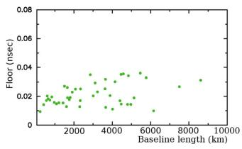
**Figure 7.** Floor of the regression model of the dependence of rms(VLBI–GPS) of RG =  $\sqrt{\text{rms}_{g1}^2 + \text{rms}_{g2}^2}$  for all VLBA baselines as a function of the baseline length.
