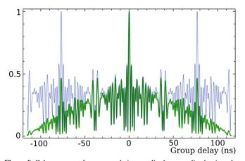
**Figure 9.** Coherent sum of cross-correlation amplitude, normalized to its value at the maximum as a function of group delay shift with respect to the maximum for VGaPS observing sessions. The thick green line shows result of processing with PIMA. The thin blue line shows results of processing with AIPS. The pattern of the thin blue line repeats with a period of 76.923 ns.
