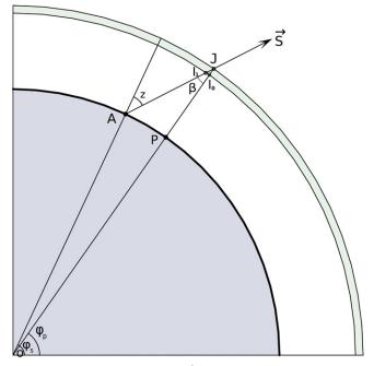
**Figure 5.** Ray traveling from source  $\vec{s}$  to antenna *A* pierces the top of the ionosphere in the point *J* and the bottom of the ionosphere in the point *I*. The ionosphere is considered a thin layer. *P* is the point on the Earth's surface beneath the ionosphere piercing point *J*.
