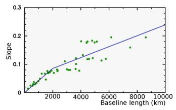
**Figure 8.** Slope of the regression model of dependence of rms(VLBI-GPS) of  $RG = \sqrt{rms_{g1}^2 + rms_{g2}^2}$  for all VLBA baselines as a function of the baseline length. The straight lines show a linear approximation of the slope for two ranges of the baseline length: below and over 2000 km.
