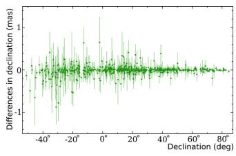
Figure 11. Systematic differences  $\Delta\delta(\delta)$  in source coordinate estimates between solutions using group delays derived by PIMA with SNR cutoff 10 and by AIPS. (A color version of this figure is available in the online journal.)
