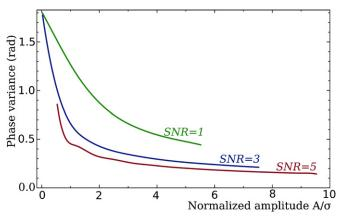
**Figure 2.** Variance of fringe phase as a function of the normalized amplitude  $A/\sigma_n$  in the presence of a signal with given SNR.
