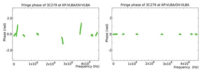
Figure 4. Residual fringe phases (radians) before (left) and after (right) applying bandpass calibration in experiment bp125b. (A color version of this figure is available in the online journal.)
