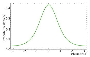
**Figure 3.** Probability density distribution of fringe phase with SNR = 1. (A color version of this figure is available in the online journal.)
